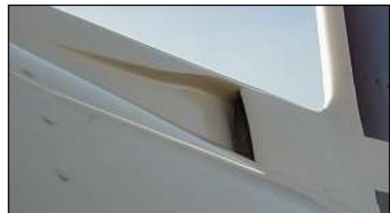
Fig.1: NACA air inlet – J-HangarSpace, 2015.
