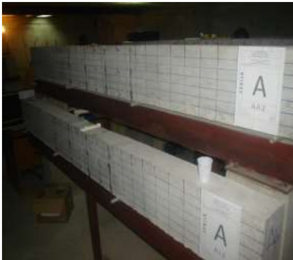
Fig. 3c: Beams treated on shrinkage [3]
